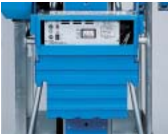
Removable battery box features separate compartments for the battery and charger.
